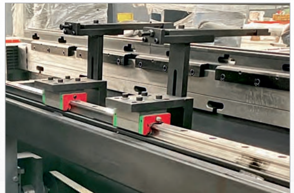
Back gauge finger movement in Z Axis on LM guide to maintain the parallelism across the table.
