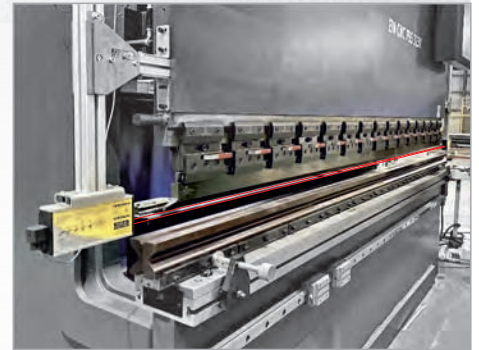
Laser beam operator safety Integrated with press brake controller
